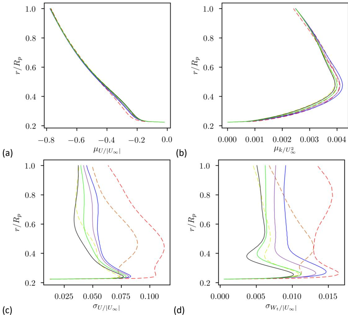
Figure 8 - Radial variation of the circumferential: (a) mean axial velocity; (b) mean turbulent kinetic energy; (c) standard deviation of the axial velocity; (d) standard deviation of the tangential velocity. Sailplane deflection lines: undeflected, —; -5°, —; -10°, —; -15°, —; +5°, -.-; +10°, -.-; +15°, -.-.
