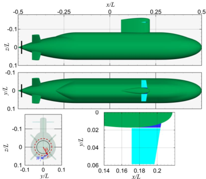
Figure 1 - DST Group BB2 generic submarine geometry, with the body-fixed coordinate system and the cylindrical coordinate system shown on the  $y$ - $z$  plane. The outer edge of the BB2 propeller, at the nominal wake plane, is shown with the thick black vertical line. The moveable sailplane section (starboard-side) is shown in light blue. The fixed portion (headbox) of the sailplane is shown in dark blue.
