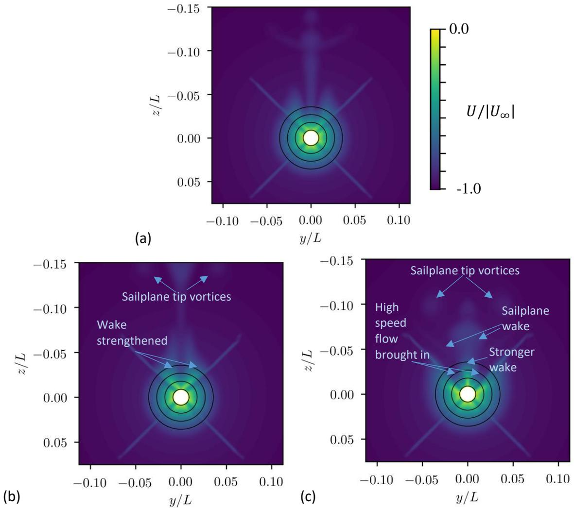
Figure 6 - Contours of the axial velocity ( $U$ ) at the nominal wake plane for sailplane deflections: (a) undeflected; (b)  $-15^\circ$ ; (c)  $+15^\circ$ . The black concentric rings are at a radius of  $0.25R_p$ ,  $0.5R_p$ ,  $0.75R_p$  and  $1.0R_p$ .
