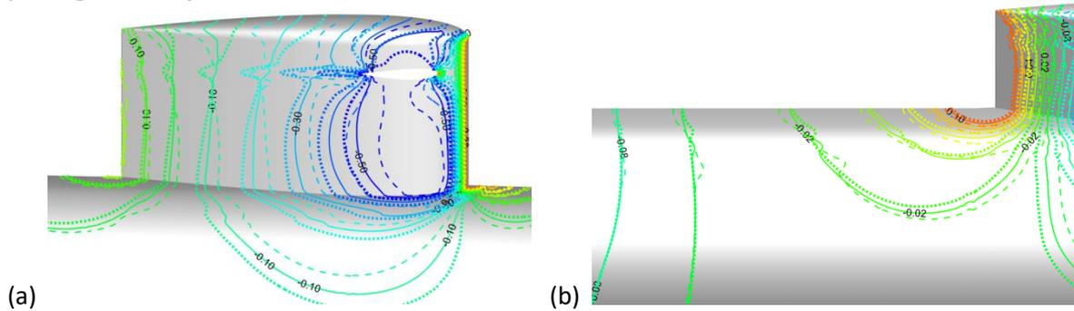
Figure 5 - Contours of the pressure coefficient for the sailplanes: undeflected, solid lines; +10° deflection, dotted lines; -10° deflection, dashed lines. Views: (a) sail region (sailplane fixed root position shown in white); (b) hull downstream of the sail.
