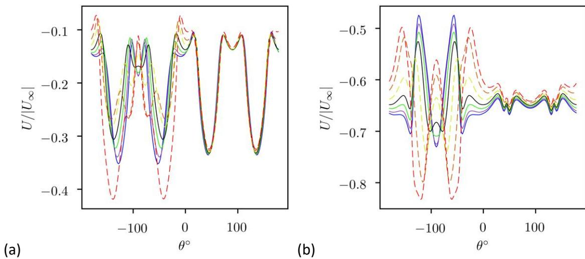
Figure 7 - Circumferential variation of the axial velocity at the propeller plane at a radius of: (a)  $0.25R_p$ ; (b)  $0.75R_p$ . Sailplane deflection lines: undeflected, —;  $-5^\circ$ , —;  $-10^\circ$ , —;  $-15^\circ$ , —;  $+5^\circ$ , —;  $+10^\circ$ , —;  $+15^\circ$ , —. Sail located at  $\theta = -90^\circ$ .
