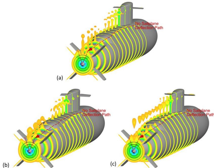
Figure 4 - Slices perpendicular to the centreline of the BB2 geometry showing contours of the streamwise velocity component. Contours cropped at 95% of the freestream speed to indicate boundary layer thickness. Sailplanes deflections: (a) undeflected; (b) leading edge up,  $+10^\circ$ ; (c) leading edge down,  $-10^\circ$ .
