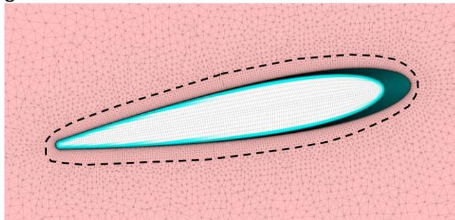
Figure 3 - Cut through a grid in the sailplane region. The dashed black line indicates the region where the Pointwise T-Rex tool recombines triangular cells to triangular prisms or hexahedra for boundary layer resolution.
