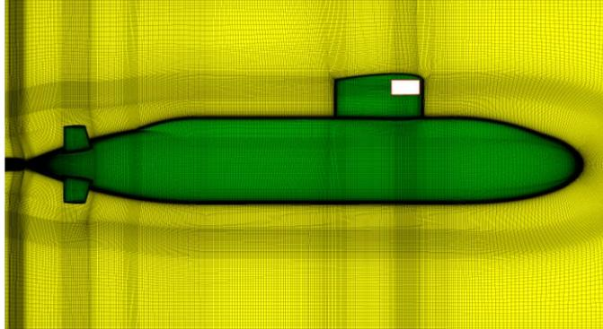
Figure 2 - Structured inner grid. The white rectangular region with a red border denotes the sailplane grid region.
