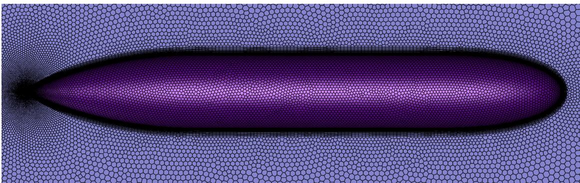
Figure 3: Mesh model of the axisymmetric bare hull Joubert geometry.
