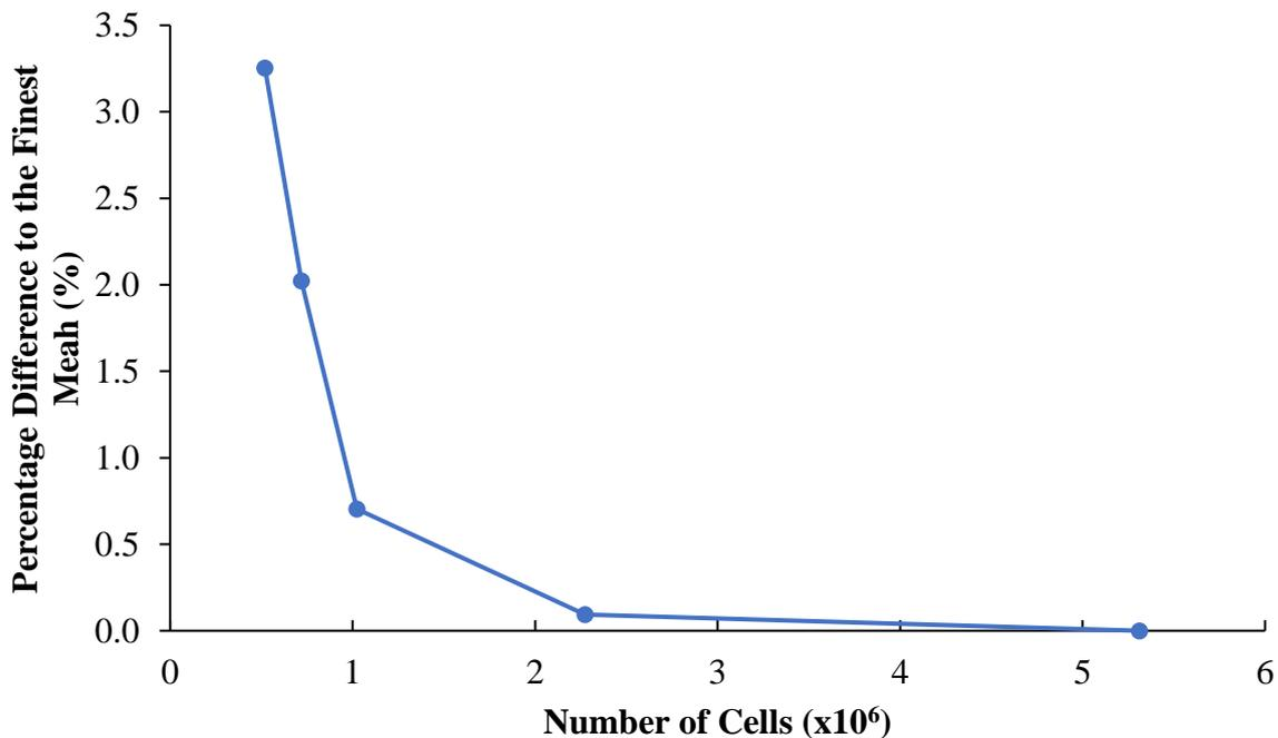
**Figure 4: Grid independent study - percentage difference in the predicted drag compared to the finest 7.1 million cell simulation solution.**
