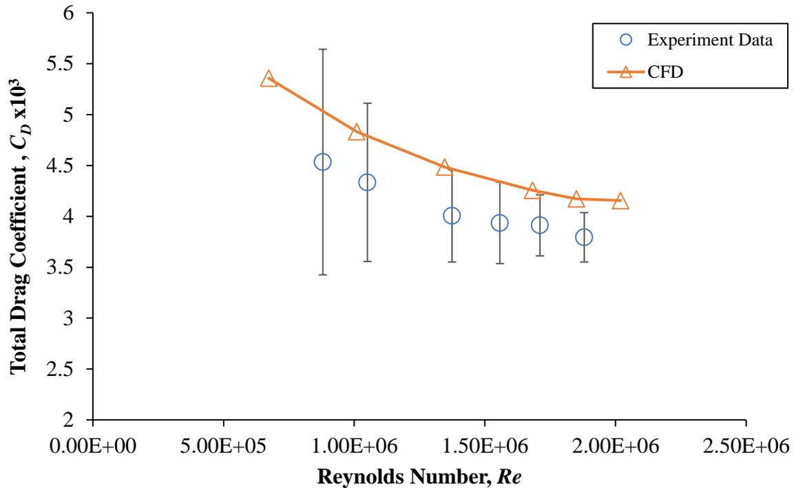
Figure 5: CFD predicted drag coefficients and experimental measurements [16] for the Joubert bare hull geometry in straight line tests, with error bars of maximum 23 % and minimum of 5%.
