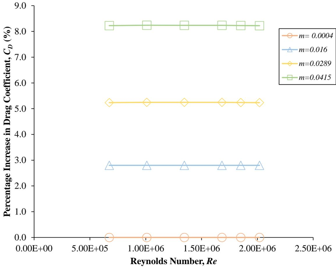
Figure 7: Percentage increase in drag coefficient,  $C_D$ , as a function of Reynolds Number,  $Re$ , for different blockage parameter ratios,  $m$  when compared to the largest blockage parameter ratio,  $m=0.0001$
