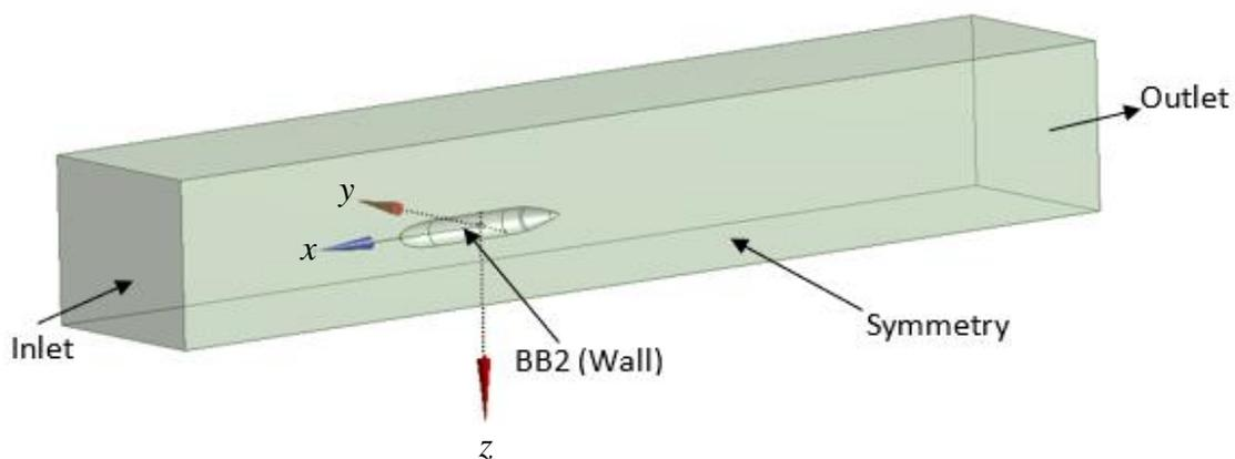
Figure 2: Computational fluid domain with coordinate system.
