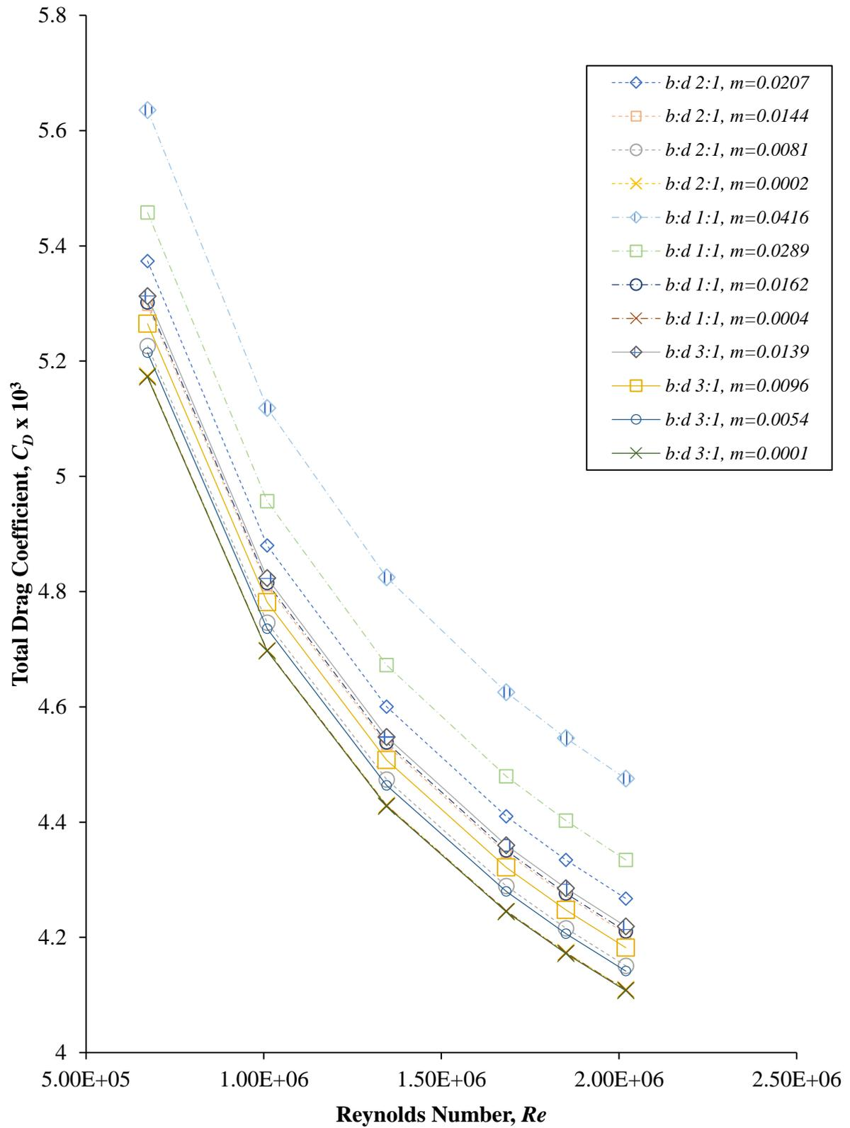
Figure 6: Total drag coefficient,  $C_D$ , as a function of Reynolds Number,  $Re$  for different domain ratios ( $b:d$ ) and blockage parameter ratios,  $m$ .
