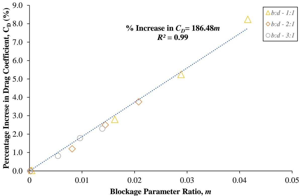
**Figure 8: Empirical correction formula for the increase in drag coefficient,  $C_D$ , when compared to the largest domain at each blockage parameter ratio,  $m$ .**
