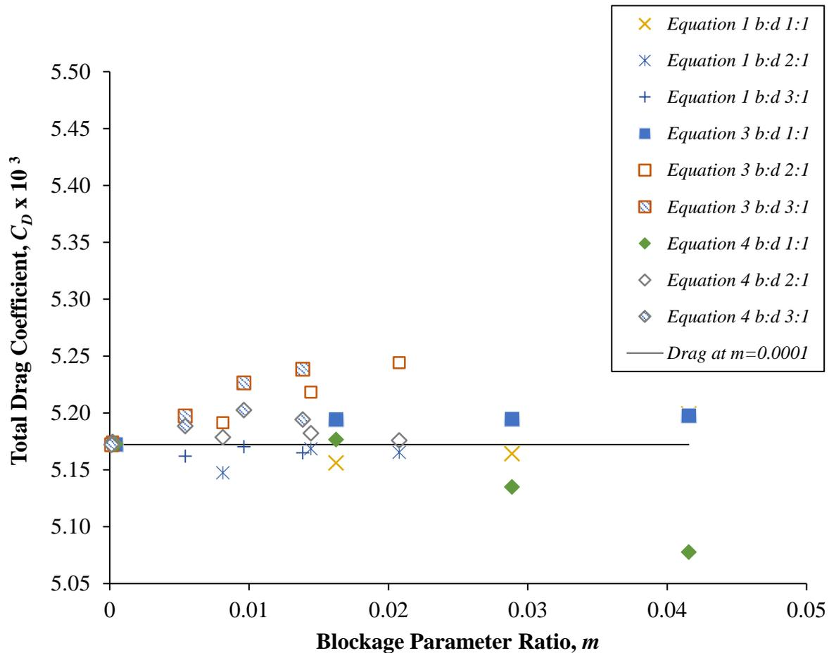
Figure 9: Total drag coefficient,  $C_D$ , predicted against blockage parameter ratio,  $m$ , at a Reynolds number,  $Re$ , of 0.6 million using different correctors.
