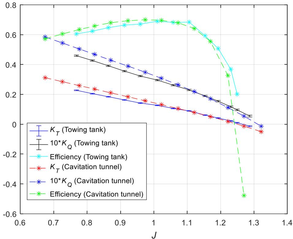
Figure 7 - Efficiency ( $\eta$ ), thrust coefficient ( $K_T$ ) and torque coefficient ( $K_Q$ ) plotted against advance coefficient ( $J$ ) values for the towing tank experiment and cavitation tunnel data [10].
