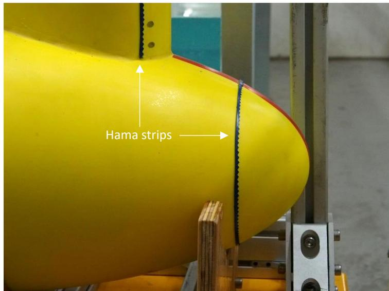
Figure 4 - Placement of Hama strip at the nose ( $x/L = 5\%$ ) and the sail ( $x/L = 10\%$ ).
