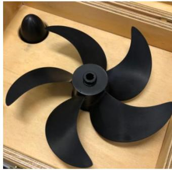
Figure 1 - DSTG 115-1 propeller with 0.15 m diameter.
