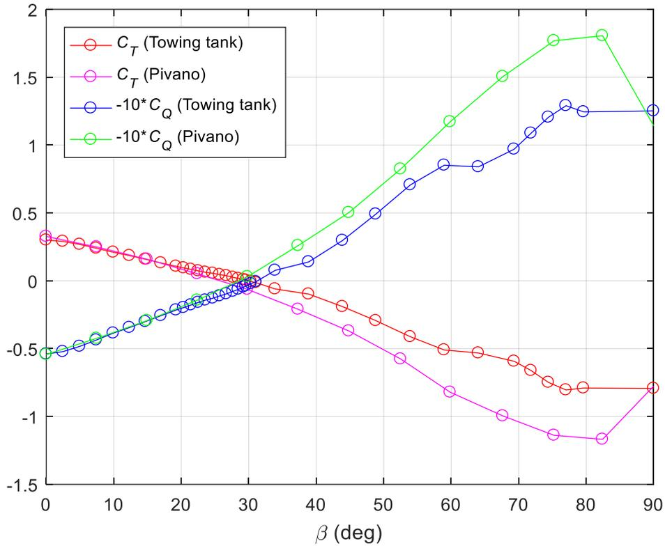
Figure 8 - Experimentally obtained non-dimensional thrust coefficient ( $C_T$ ) and torque coefficient ( $C_Q$ ) vs. advance angle ( $\beta$ ) for first propeller quadrant. Results compared with data from Pivano [2].
