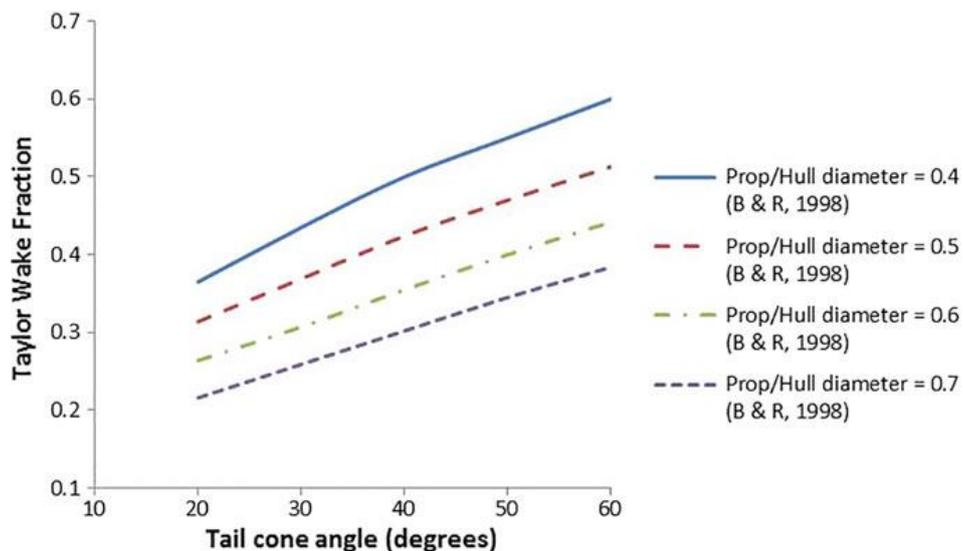
Figure 5 - Taylor wake fraction for underwater vehicles based on prop/hull diameter ratio and tail cone angle [8].
