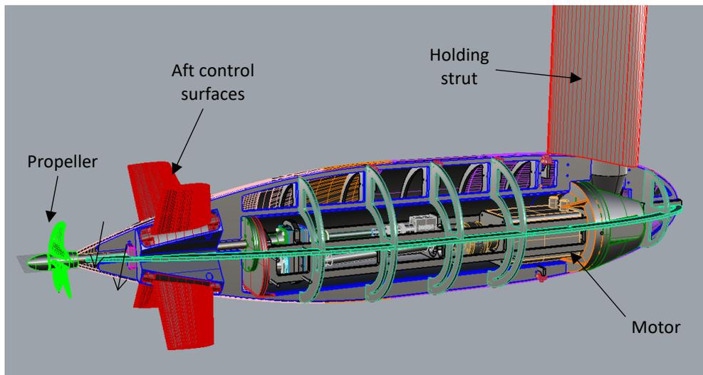
Figure 2 - Schematic drawing showing internal layout and external shape of the experiment model.
