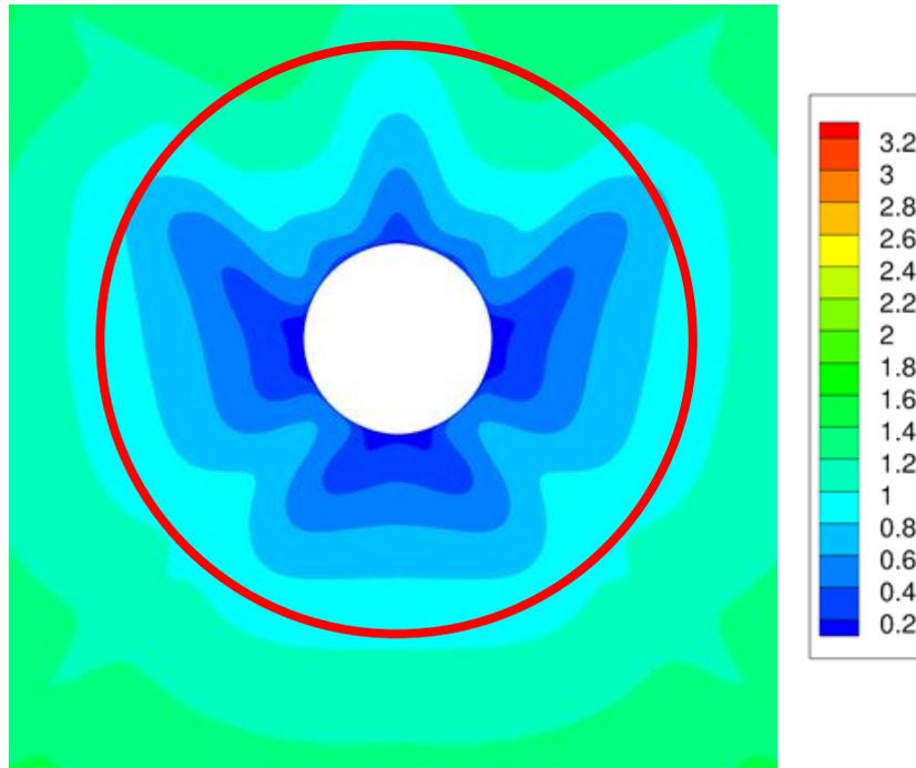
Figure 6 - Axial velocity gradient at the propeller plane for the BB2 submarine with a free stream velocity of 1.6 m/s. The red circle represents  $0.7D$  for velocity prediction.
