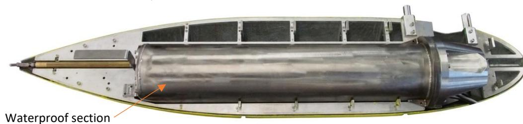
Figure 3 - Cross section of the towing tank model with waterproof section.
