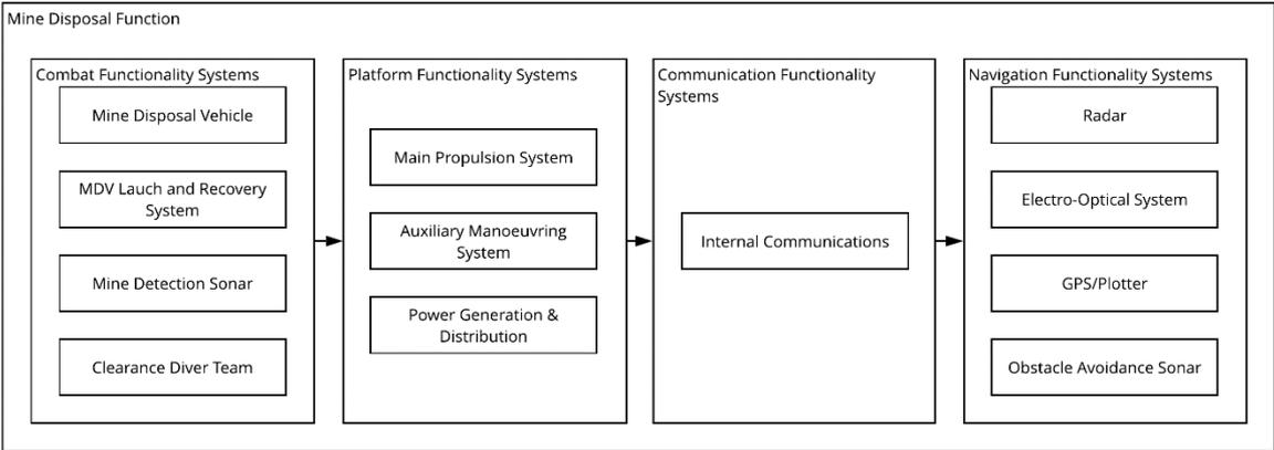
Then, using the outcomes of the bottom-up derived availability analyses of the physical subsystems that contribute to the overall function, an availability for the top-level function may be derived, shown via the availability block diagram in Figure 4.
