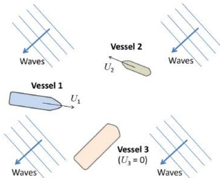
Figure 2 Multi-vessel SSE operational setup by Nielsen et al. [14]. Reprinted from Applied Ocean Research, Vol 83, U. D. Nielsen, A. H. Brodtkorb, and A. J. Sørensen, Sea state estimation using multiple ships simultaneously as sailing wave buoys, Page 71, Copyright (2019), with permission from Elsevier.
