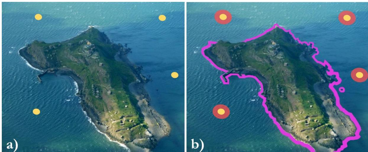
Figure 2 **a)** Initial SSE target locations (yellow dots) in an example environment. **b)** Target location attraction radii (orange shadows) and obstacle repulsion radii (pink shadow). The image has been modified from a picture taken by Gyula Péter, available on Wikipedia Commons [21].
