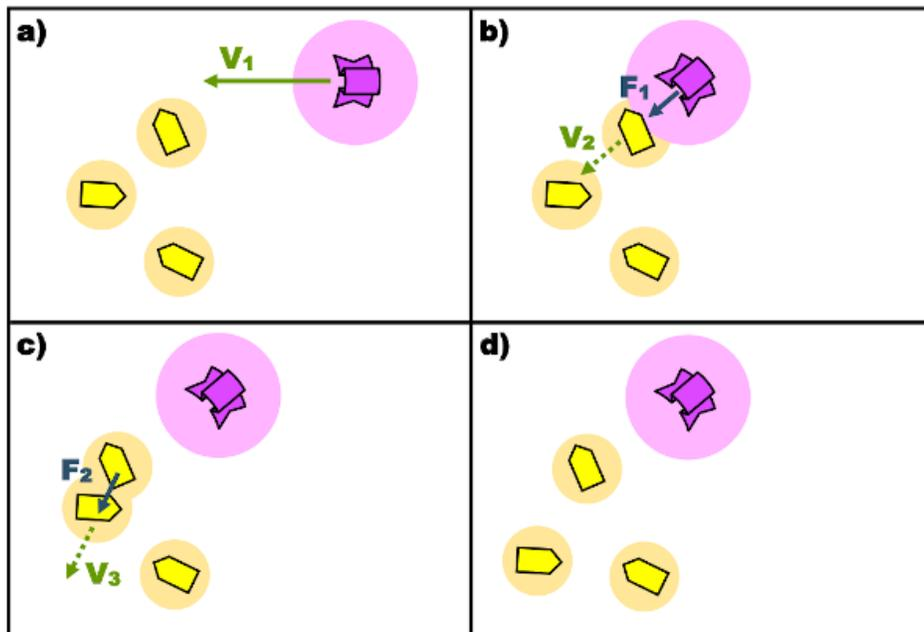
Figure 1 Repulsion radii between shepherd (pink) and swarm agents (yellow) are shown. **a)** Shepherd moves with initial velocity  $V_1$ . **b)** Swarm agent within repulsion radius of shepherd so force  $F_1$  imparted on it, then agent moves away with velocity  $V_2$ . **c)** Swarm agent within swarm agent repulsion radius so force  $F_2$  imparted on it, then it moves away with velocity  $V_3$ . **d)** Final position of agents.
