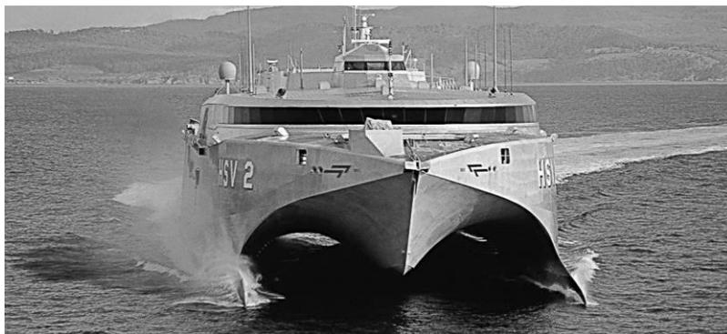
*Figure 1 A Photograph of Incat HSV-2 Incat High-speed Wave-piercing catamaran [hull 061] during sea trials [1]*
