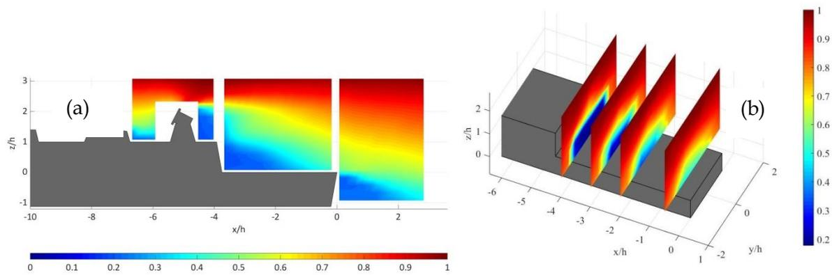
Figure 7: Normalised velocity contours over (a) NATO-GD and (b) SFS2
