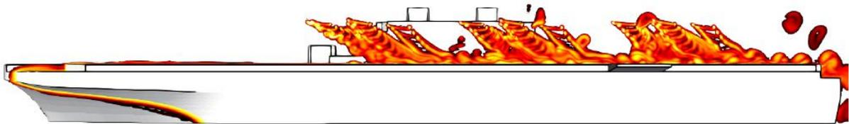
Figure 5: Vorticity magnitude on a plane through the port landing spots on the LHA ship with three tandem rotor helicopters
