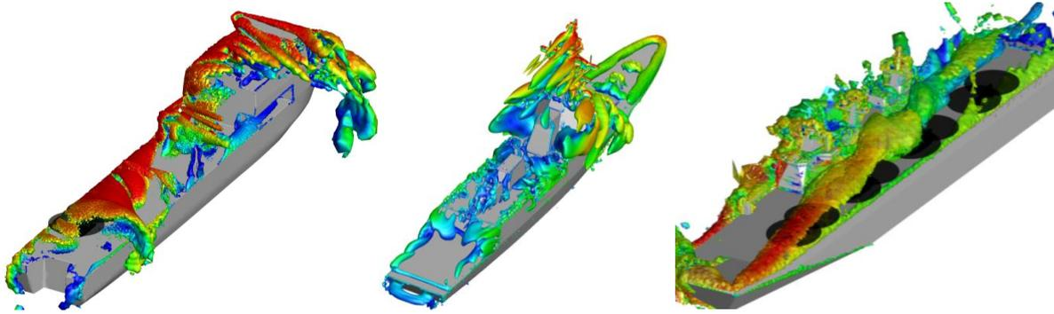
Figure 2: Example of few CFD ship airwake from DST Group database
