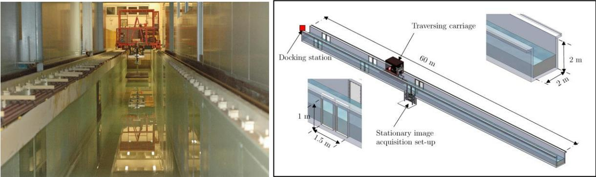
Figure 6: Extreme Air Sea Interaction (EASI) facility at the University of Melbourne
