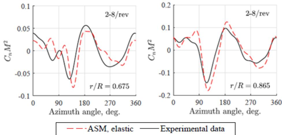
Figure 4: 2-8/rev vibratory components of normal force coefficient as a function of azimuth angle at two spanwise stations on the UH-60A rotor in forward flight at an advance ratio of 0.368. ASM simulation results compared to experimental data.
