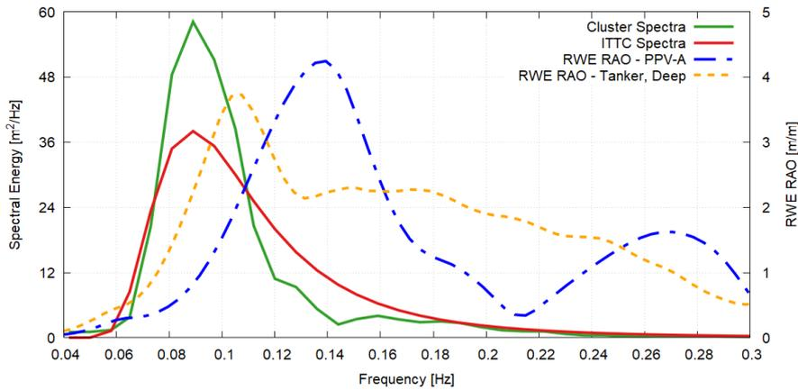
**Figure 10: Comparison of Cluster and ITTC Spectra Against Relative Wave Elevation RAOs**
