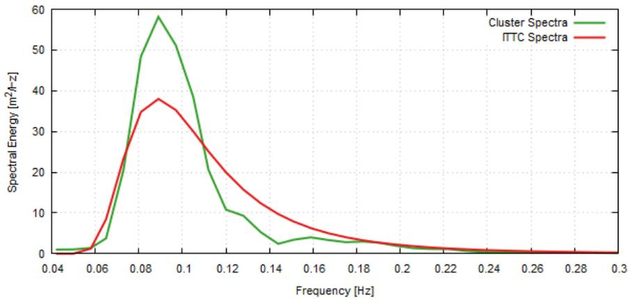
Figure 8: Comparison of Ross Sea, Sea State 7, Spectrum 1 with corresponding ITTC Spectra
