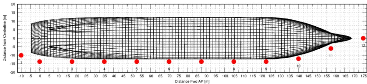
Figure 3: Example of Locations of Relative Wave Elevation Calculations, Plotted Against Hull Mesh to Waterline
