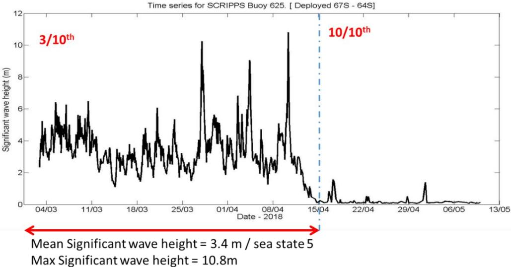
Figure 1: Significant Wave Height Data from Wave Buoy Deployed in Ross Sea Marginal Ice Zone, March / April 2018
