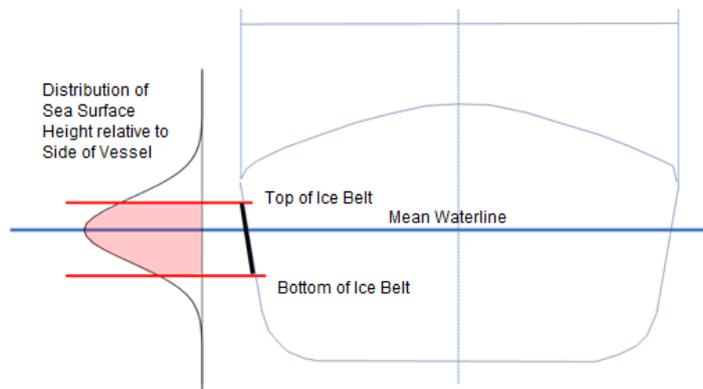
Figure 4: Normally Distributed Relative Wave Elevations
