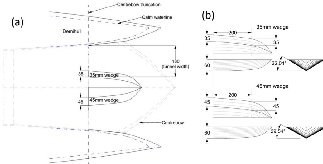
**Figure 6:** Showing (a) the horizontal faces that occupy 20% and 25% of the tunnel width on a plane 70 mm above the waterline for the 35 mm and 45mm wedge respectively, and (b) the lines and principal geometry of the 35mm and 45mm wedge sections.
