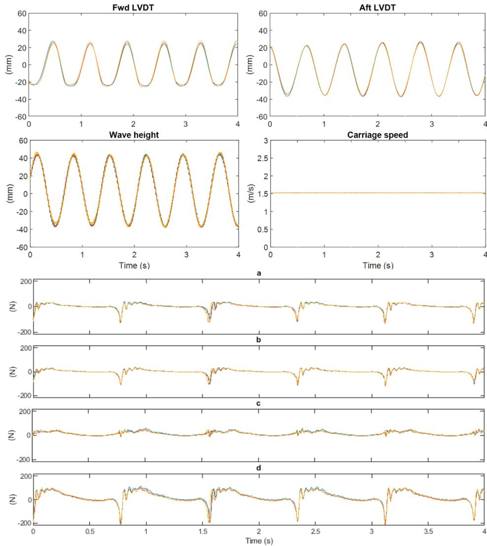
**Figure 8:** Showing 3 run results of condition 1. The results include the aft and Fwd LVDTs, static wave height sensor, carriage speed, and the measured forces of (a) the port side load cell, (b) starboard load cell, (c) Aft load cell, and (d) The total load, e.g. instantaneous summation of the three load cell measurements.
