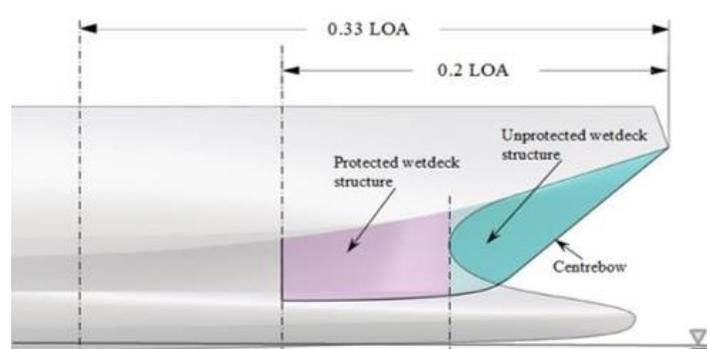
**Figure 2:** Showing the main area of interest in the design of high-speed catamarans, which is the impact loading in the vicinity of the centrebow (Swidan, 2017).
