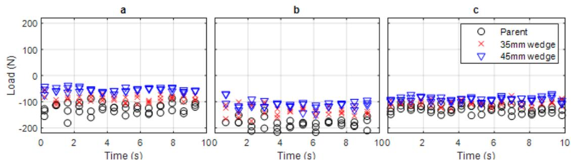
**Figure 11:** Showing all measured slam peak force magnitudes of conditions 1, 2 and 3.
