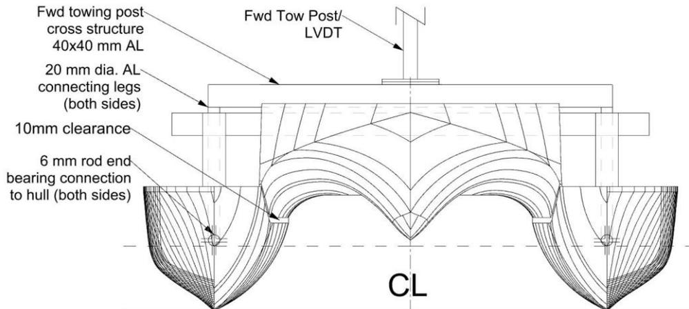
**Figure 4:** Body plan of the NPL's demihulls fitted with a generic centrebow and the forward towing configuration.
