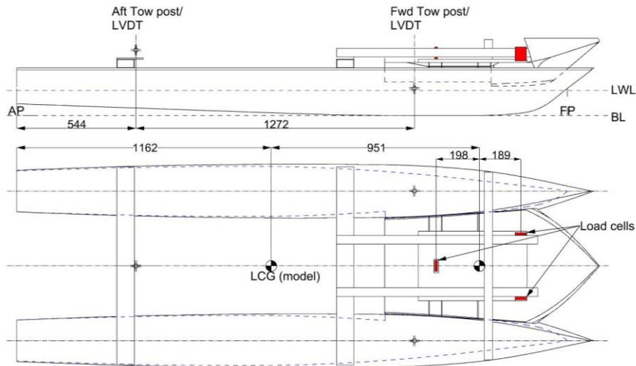
**Figure 7:** Plan and profile views of the model setup showing locations of load cells and tow posts
