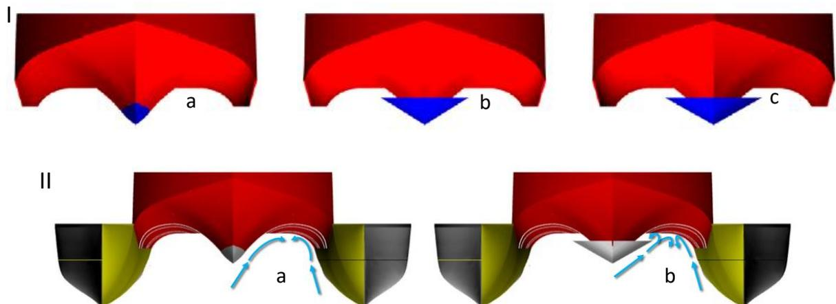
**Figure 5:** I-(a) Showing the parent centrebow; (b) 35 mm wedge fitted to parent centrebow; (c) 45 mm wedge. (a), (b) and (c) are viewed from forward and omit the demihulls. Figure 3 II-a showing the semi-entrapped flow behaviour between the parent centrebow and the demihull, (b) illustrates an early flow separation around the tip of the 35 mm wedge.
