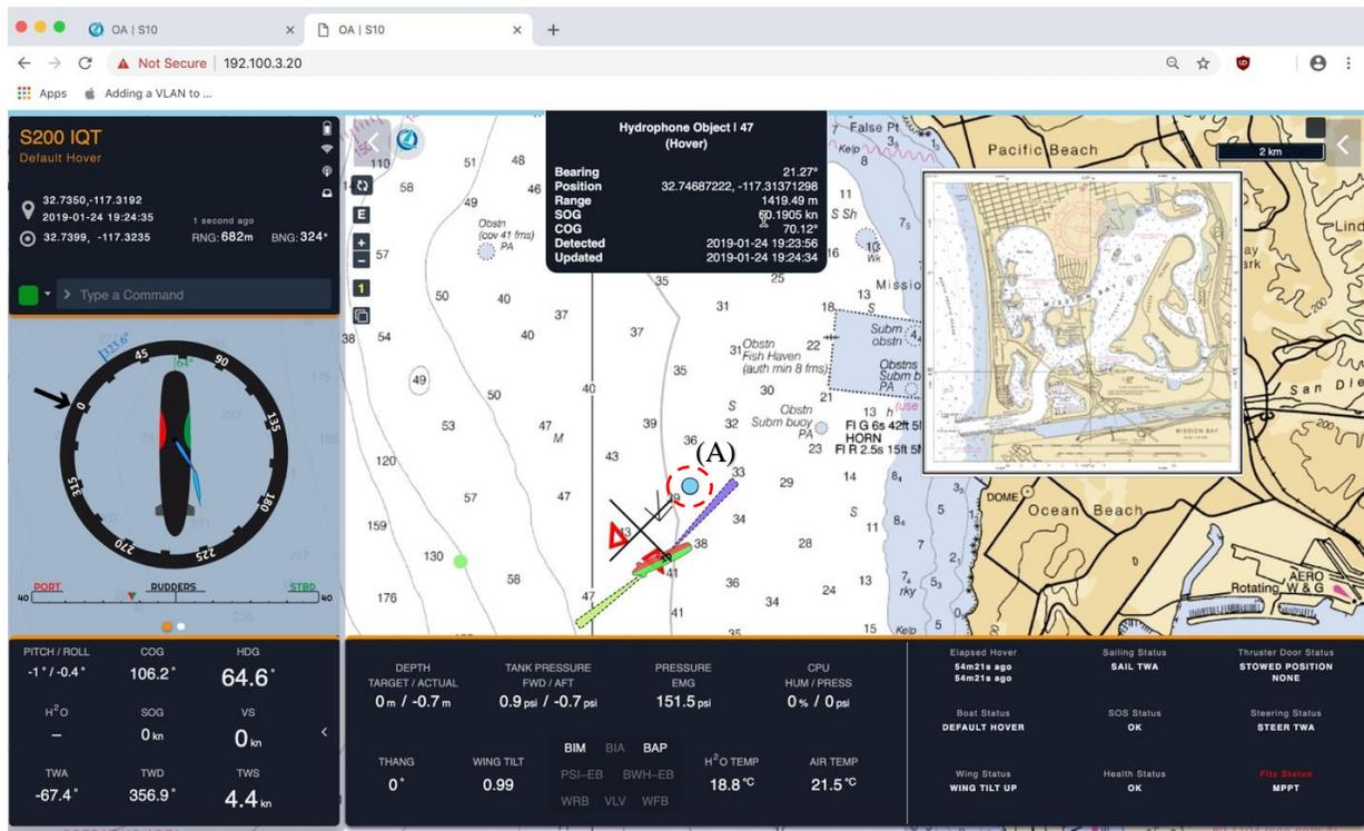
Figure 3. Location of at-sea trial showing the position of the AUSV, nearby AIS targets and the initial detection of the 500Hz target of interest (A)
