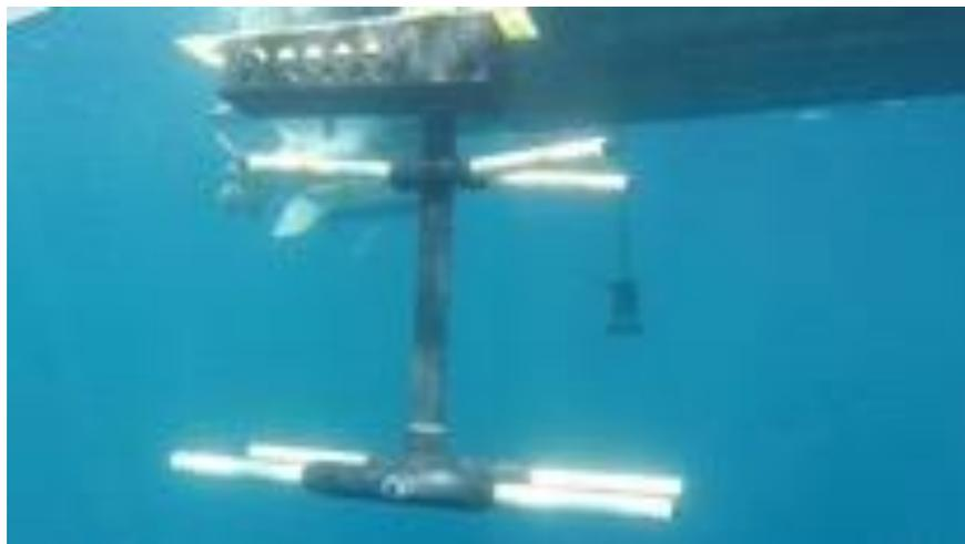
*Figure 2: The 3-D multi-hydrophone array during in-water testing*
