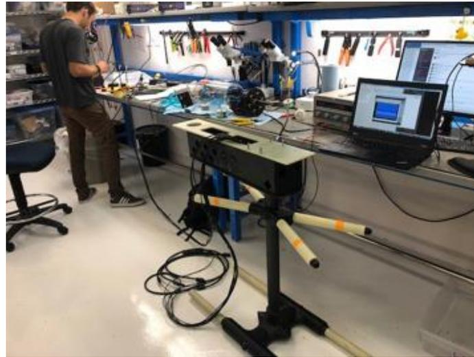
*Figure 1: The 3-D multi-hydrophone array during bench tests*
