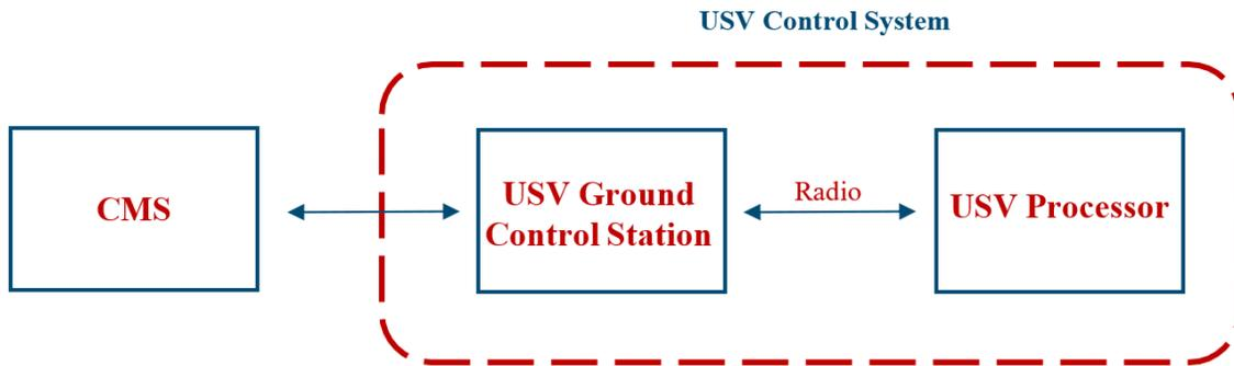
This architecture allows the CMS to send commands to the USV's ground control station, which then converts the message to a format readable by the USV processor.
