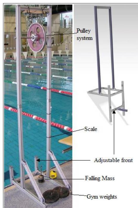
**Figure 1 – Drop tower Developed by Ryan Cavanagh in 2018 [5]**
