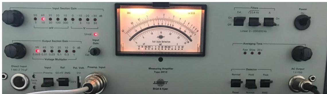
Figure 2: Measuring Amplifier used in Air Tests
