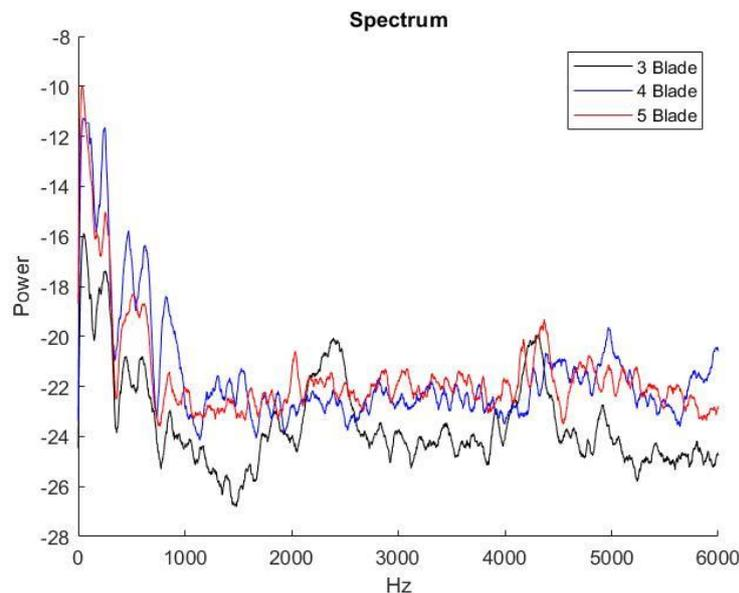
Figure 12: An overlay of the filtered spectrum of the varied propellers
