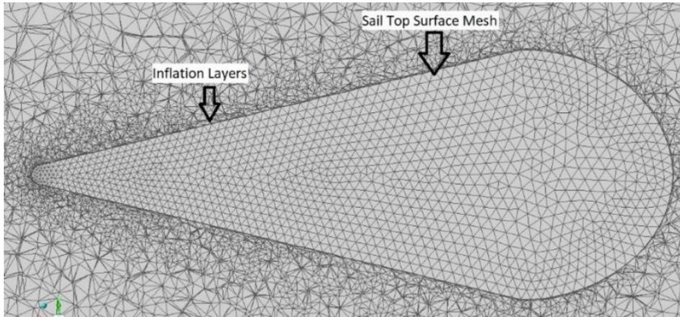
Figure 5: (b) Top view of sail mesh and inflation layers (Medium Mesh)
