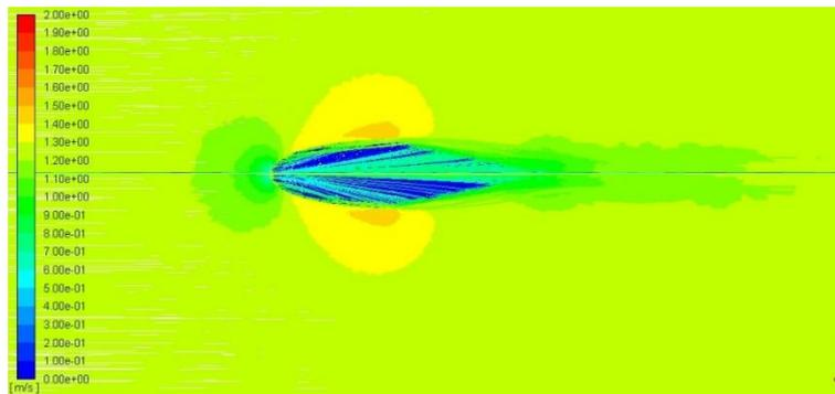
Figure 8: (c) Velocity path lines around geometry 3 at 1.25m/s, top view
