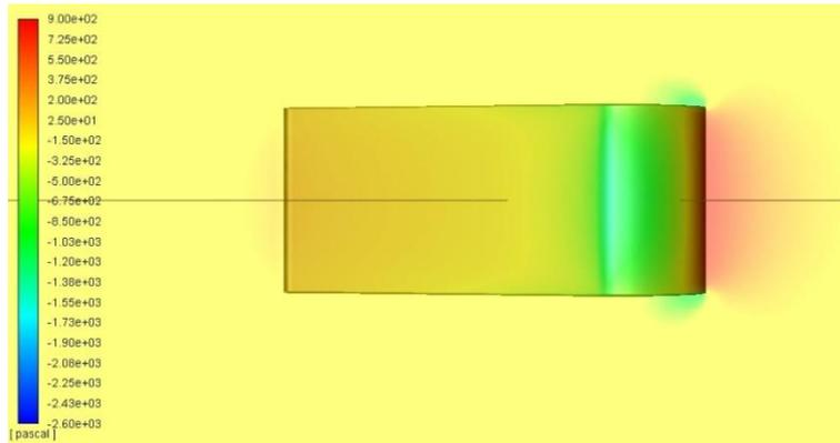
Figure 6: (b) Contours of static pressure geometry 2 at 1.25m/s, side view
