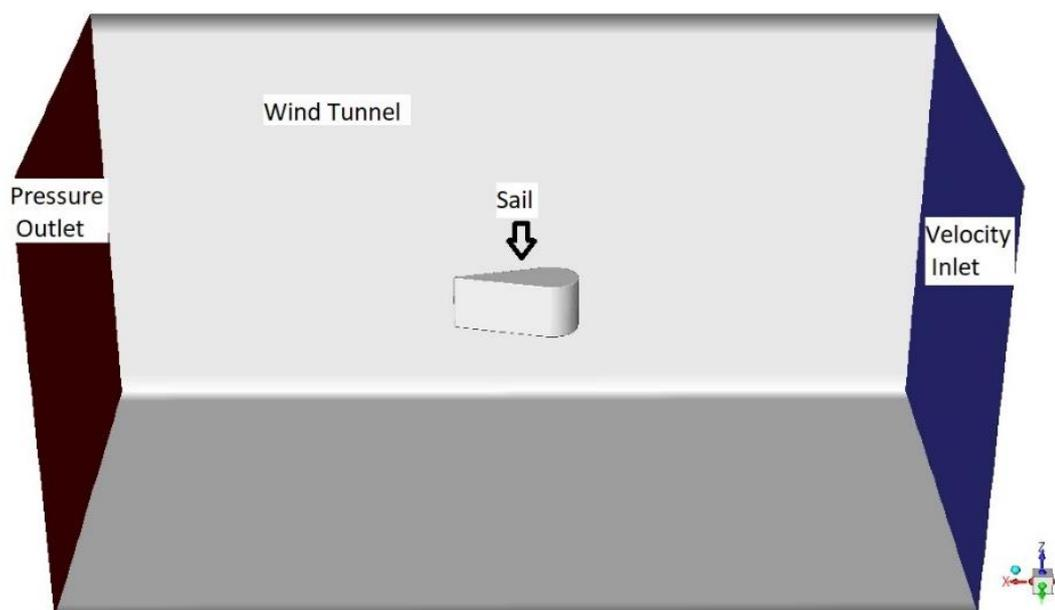
Figure 4: Display of basic setup (Front walls of wind tunnel removed for visualisation)
