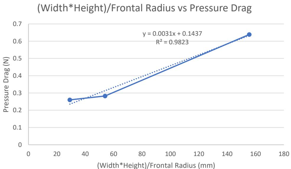
Figure 7: Graph of primary features of the geometries and the influence on the pressure drag at 1.25m/s.
