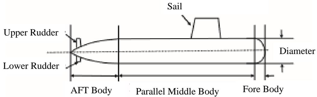
Figure 1. Side view of a generic submarine hull (Renilson, 2015).
