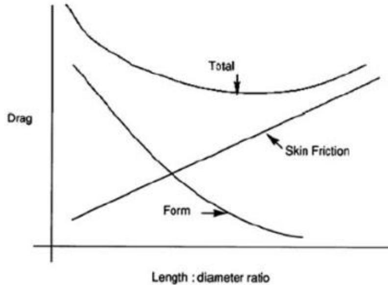
Figure 2. Graph displaying the contradicting nature of form and frictional drag (Mooresun *et al.*, 2013).
