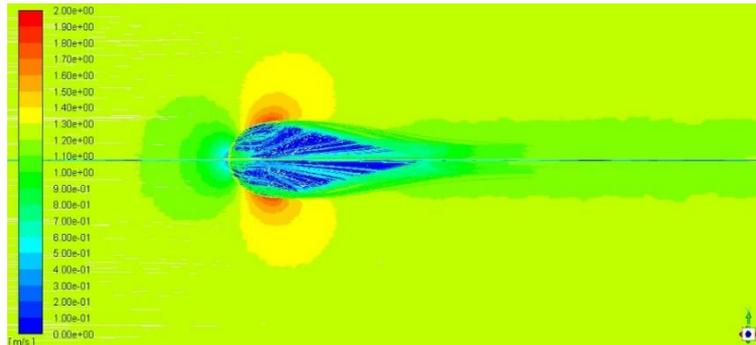
Figure 8: (b) Velocity path lines around geometry 2 at 1.25m/s, top view
