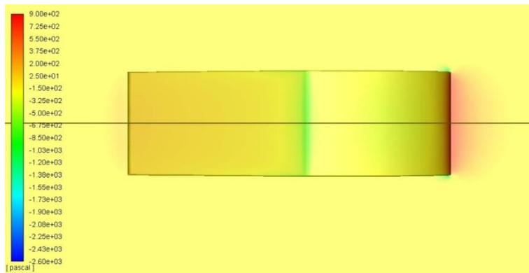
Figure 6: (c) Contours of static pressure geometry 3 at 1.25m/s, side view
