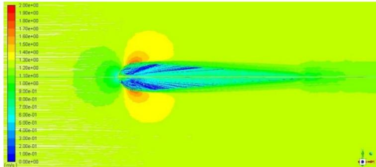
Figure 8: (a) Velocity path lines around geometry 1 at 1.25m/s, top view
