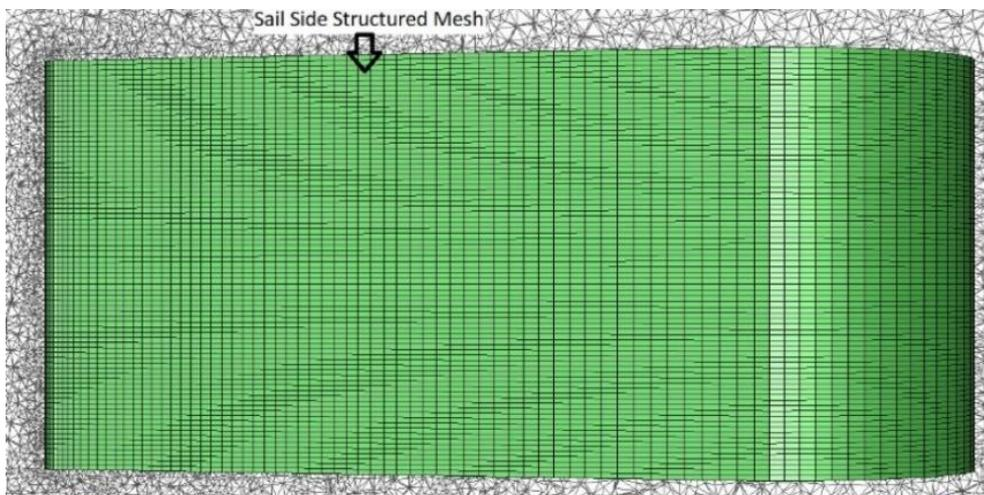
Figure 5: (c) Side view of sail structured mesh (Medium Mesh)
