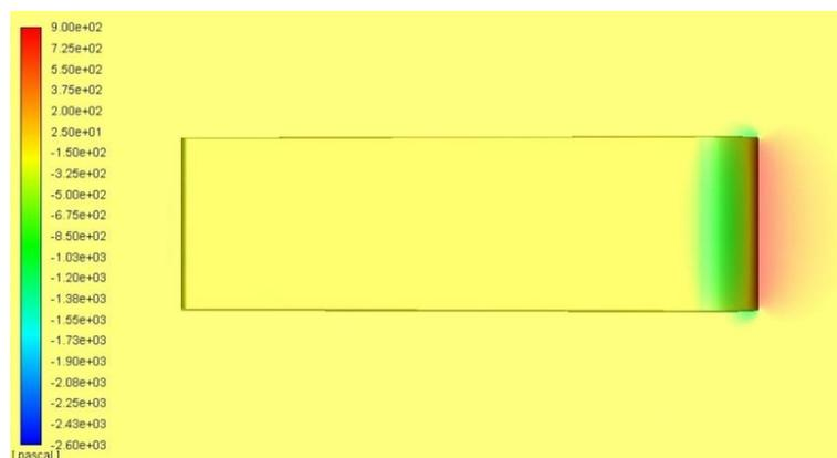
Figure 6: (a) Contours of static pressure geometry 1 at 1.25m/s, side view
