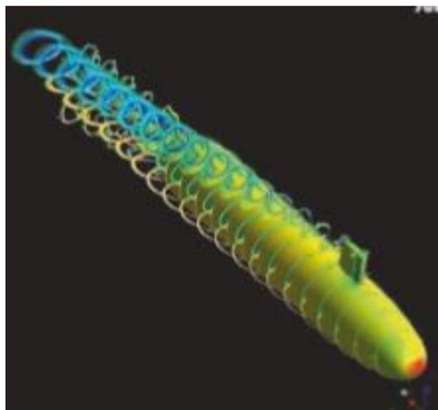
Figure 3. Flow vortices around a maneuvering submarine (Renilson, 2015).
