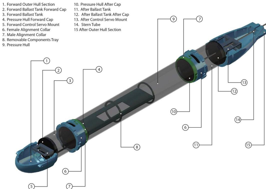
**Figure 6 – The proposed redesign for the pressure hull and depth-control system**
