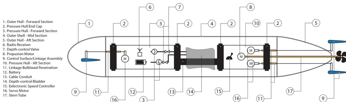
Figure 1 – Schematic diagram of SIS base kit
