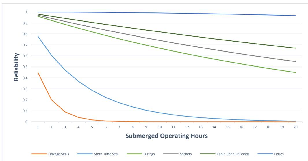
**Figure 5 - Reliability of Pressure-hull Components as a Function of Time**
