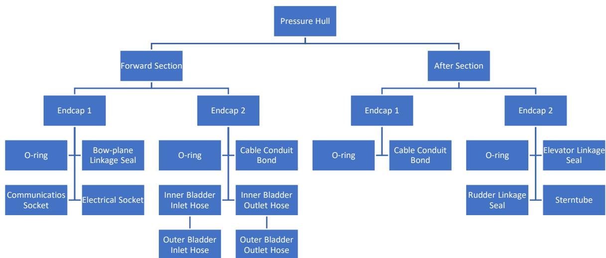
**Figure 4 - Functional Component Layout: SiS Kit Model Pressure-Hull**
