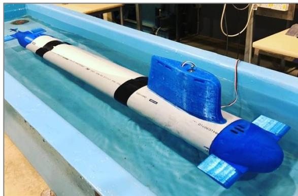
**Figure 2 – Completed base kit-model surfaced in test bath**
