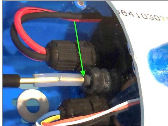
**Figure 3 – Image of the bow-plane linkage seal (leakage point indicated)**
