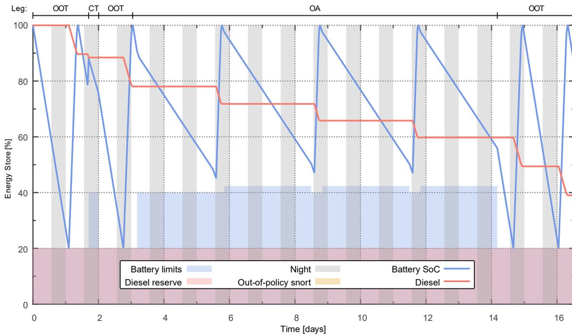
Figure 6: Evolution of energy store levels over the scenario illustrated in Figure 5, as generated by the IPSM. Mission segments depicted: Open Ocean Transit (OOT), Constrained Transit (CT) and Operational Area (OA).
