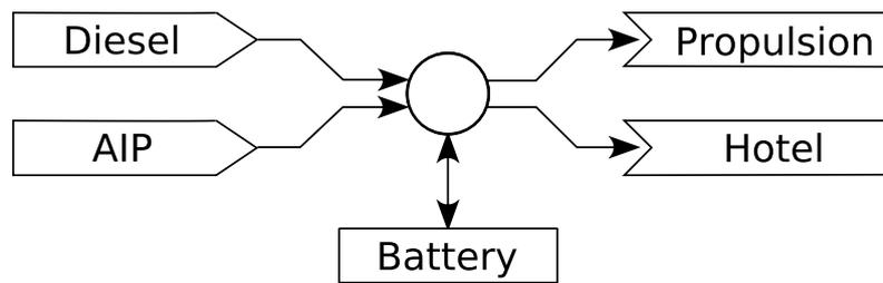
*Figure 1: Top level electrical energy producers and consumers in an IPSM platform model.*
