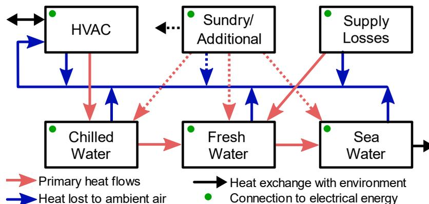
Figure 3: Structure of thermal flows for a suggested base set of platform systems. Dotted lines indicate the potential links for additional systems created using the 'Sundry/Additional' template.
