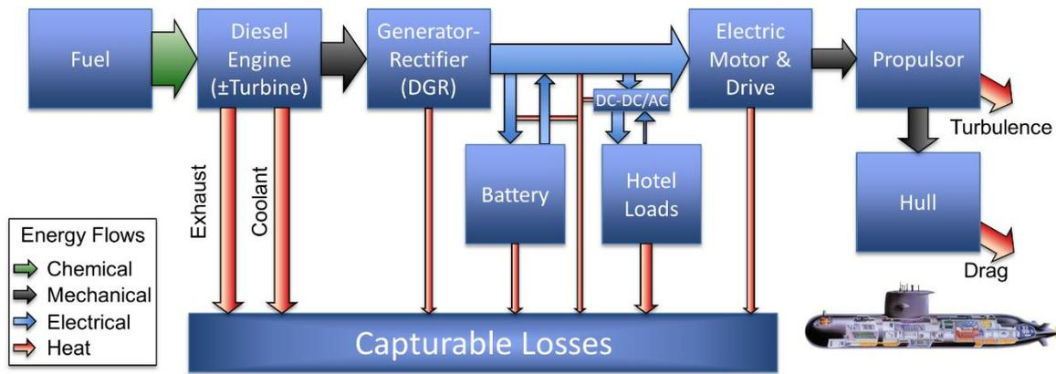
Figure 4: Sankey diagram of major energy flows in a diesel-electric submarine
