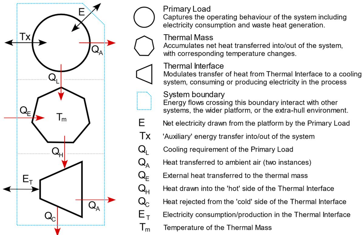
Figure 2: Schematic of energy flows for a single system
