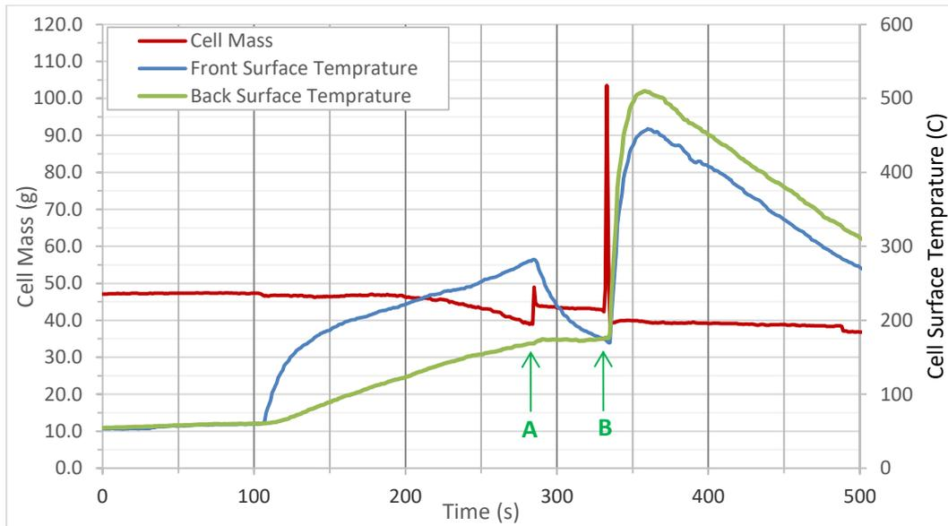
Figure 4. Mass and surface temperature behaviour resulting from heating the large surface of a lithium-ion polymer cell using a radiant burner.
