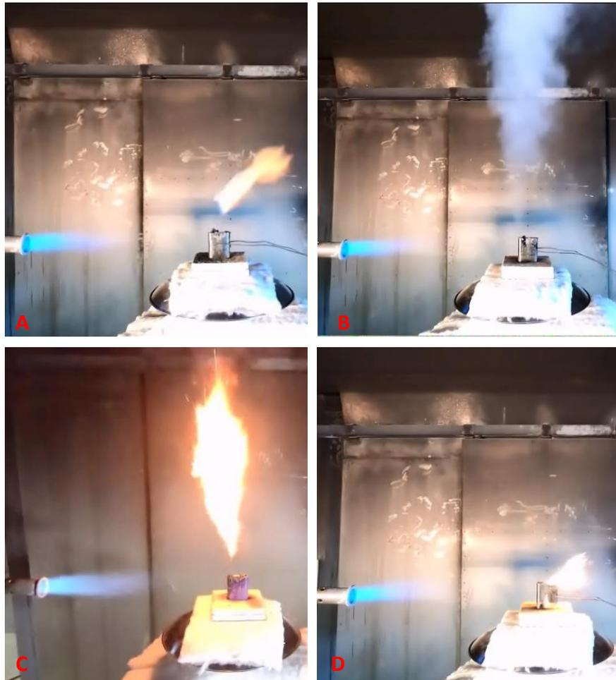
*Figure 2. Typical stages of a lithium-ion polymer battery fire test. (A) A propane burner ignites a small vented gas jet. (B) The jet develops into a rapid venting prior to ignition that extinguishes the flame and (C) then re-ignites. (D) The combustible cell internal materials and packaging continue to burn after the electrolyte is consumed.*
