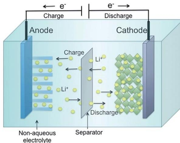
*Figure 1. The insertion of lithium ions (yellow spheres) into the anode and cathode matrices during the charging and discharging processes [9].*
