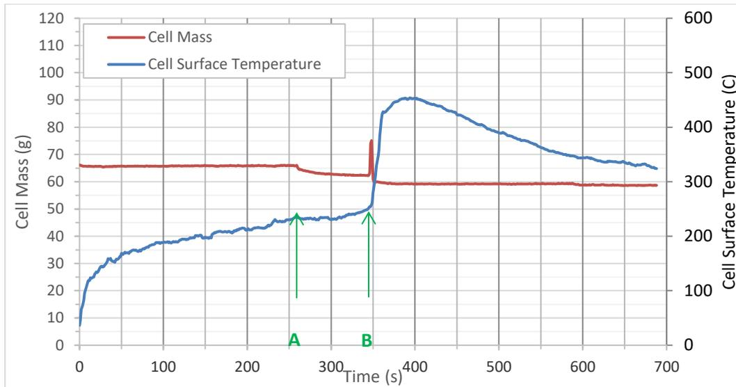
Figure 3. Mass and surface temperature behaviour resulting from heating a lithium-ion polymer cell using a side mounted propane gas burner.
