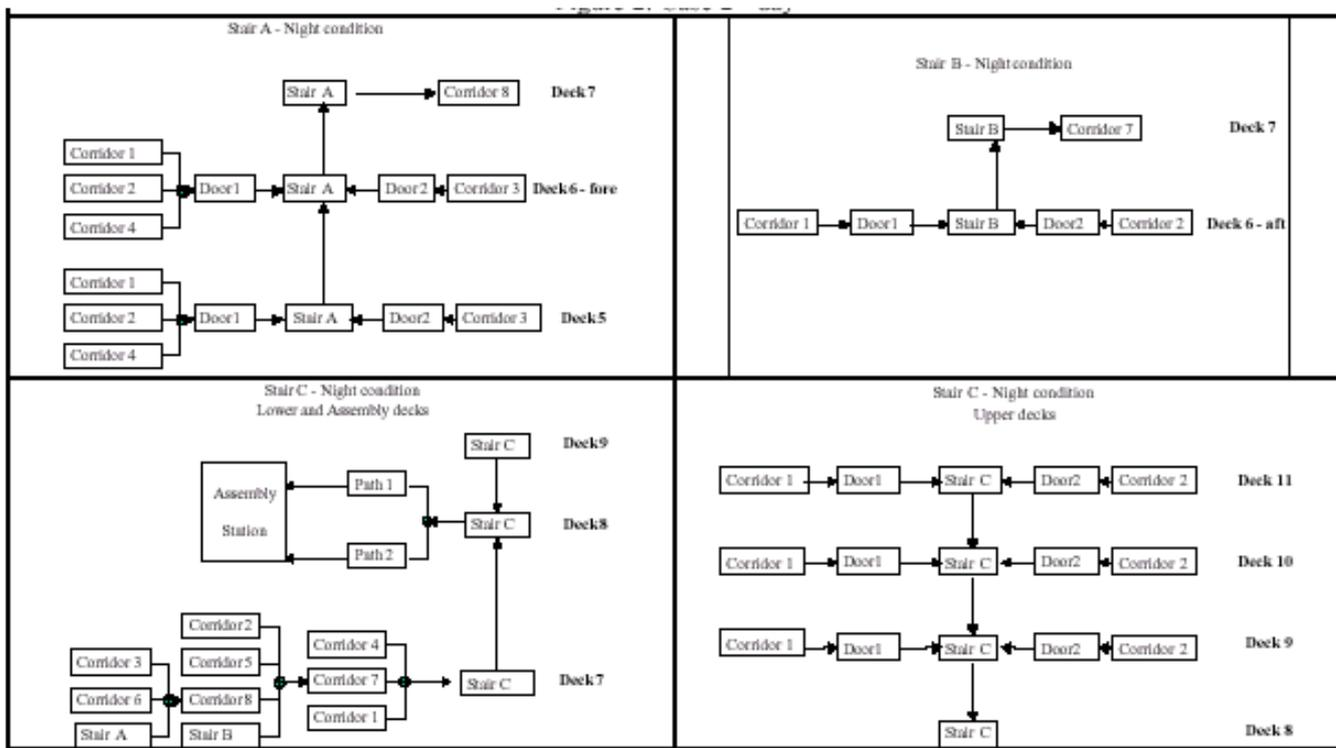
Figure 1 From MSC/1533 – Case 1 Night Case Hydraulic Representation
