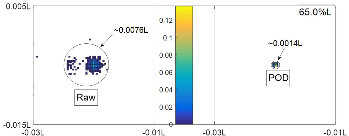
Figure 7. Probability density function (PDF) of the instantaneous vortex centre of the raw and POD-corrected velocity vectors identified by the minimum vorticity at three axial locations along the model.
