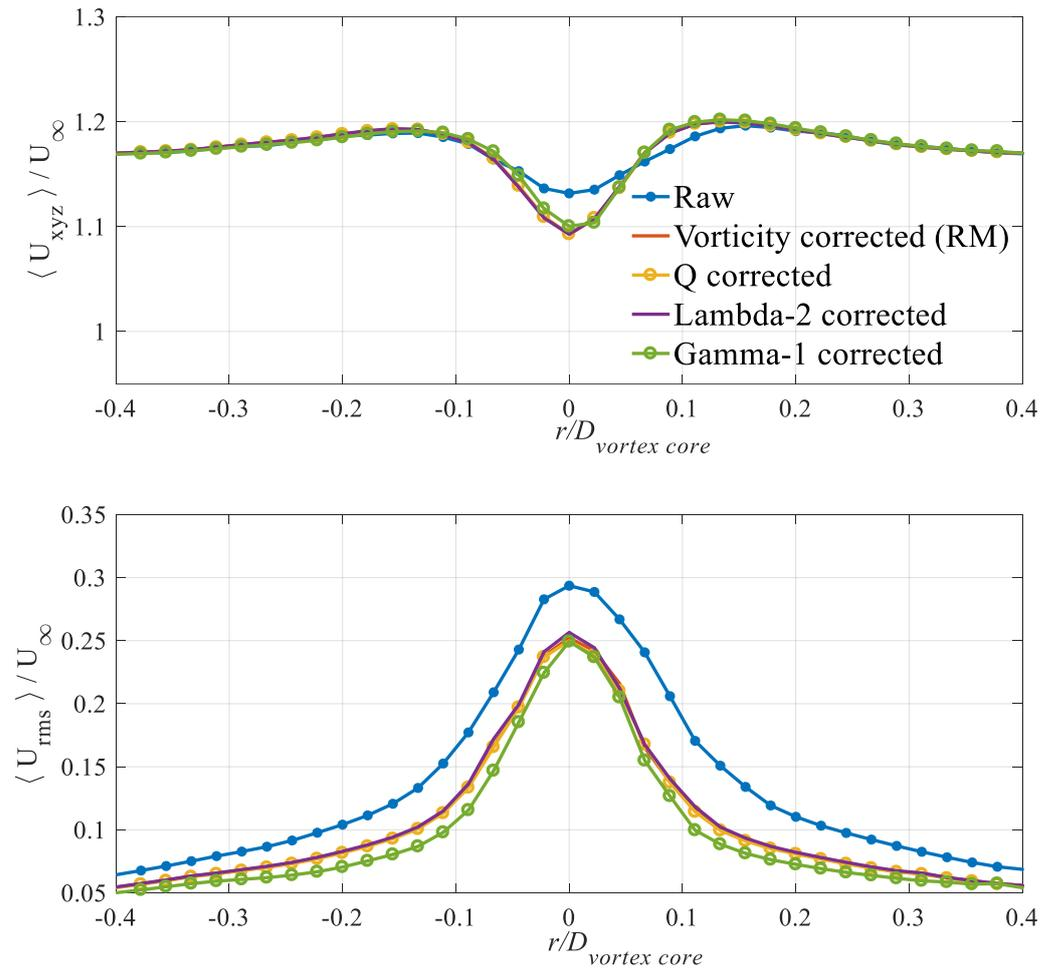
Figure 9. The normalized resultant velocity and fluctuation of raw data and meandering corrected results using different vortex identification criteria at 65.0%L.
