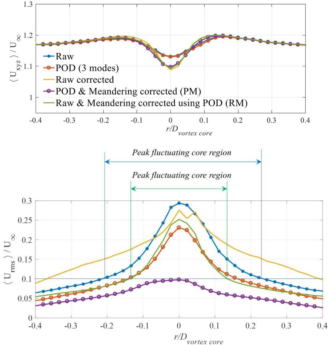
Figure 8. The normalized resultant velocity and fluctuation of Raw, POD approximated, raw corrected, POD & Meandering corrected and Raw & Meandering corrected using POD results at 65.0%L.
