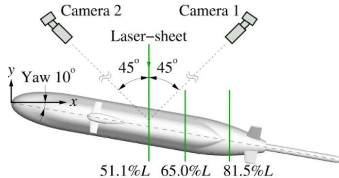
Figure 1. The BB2 generic conventional submarine model at 10° yaw and the SPIV measurement planes.
