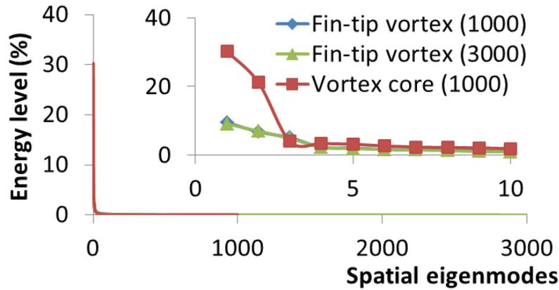
Figure 4. Contributions from the POD eigenmodes to the total energy for different cases with a particular focus on the first ten modes (1000 snapshots of the bridge fin-tip vortex, 3000 snapshots of the bridge fin-tip vortex and 1000 snapshots of the vortex core).
