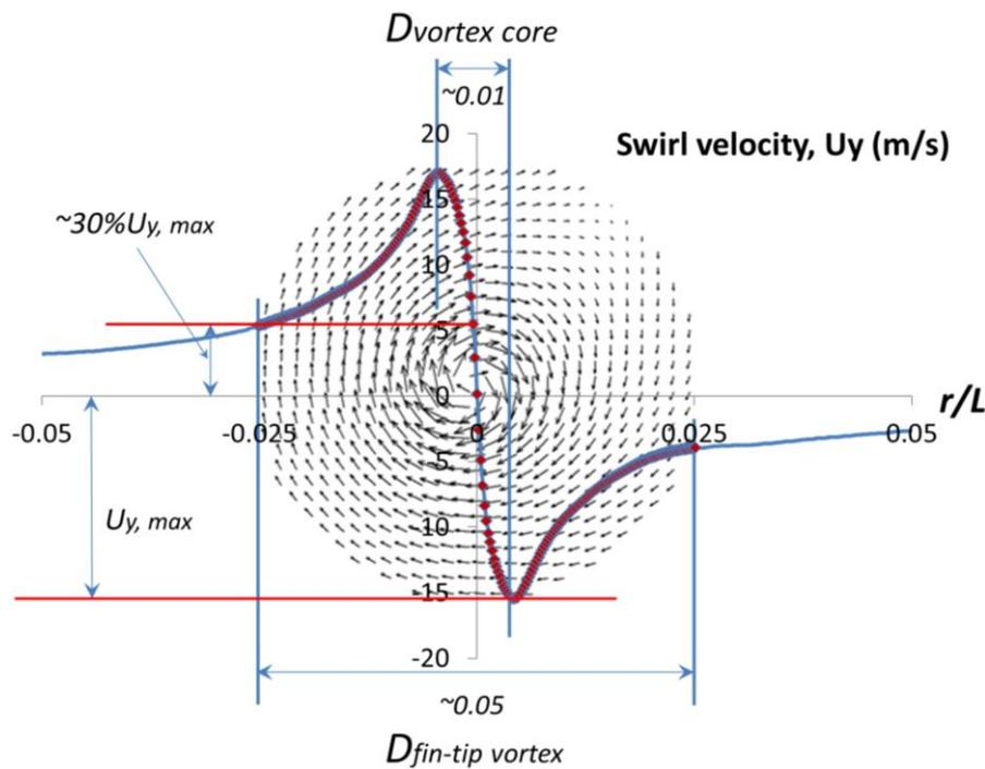
Figure 3. Swirl velocity distribution across the bridge fin-tip vortex and the selected views for POD analysis.
