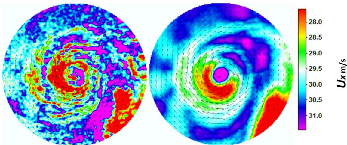
Figure 2. Left: an instantaneous velocity field of the bridge fin-tip vortex at 65% of the model length. Right: reconstruction of the same instantaneous velocity field based on the first three modes from the POD analysis. The contour levels represent the out-of-plane streamwise velocity ( $U_x$ ).
