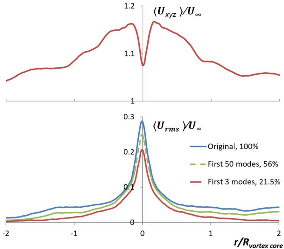
Figure 6. The normalized resultant velocity and the turbulence intensity of the original raw data, the POD approximation (first 50 modes, 56% of total turbulent energy) and the POD approximation (first 3 modes, 21.5% of total turbulent energy at 65%L).
