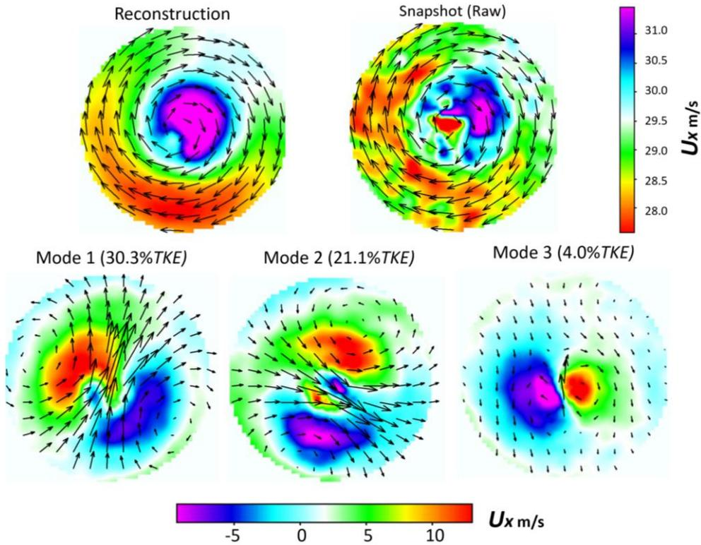
Figure 5. Top: an instantaneous velocity field of the vortex core and the reconstruction of the flow field based on the first three modes. Bottom: first three POD modes with their eigenvalues/energy level.
