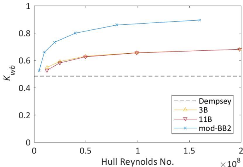
**Figure 12:** ACS efficiency variation with Reynolds Number for the appended Model 4621 hull and mod-BB2.
