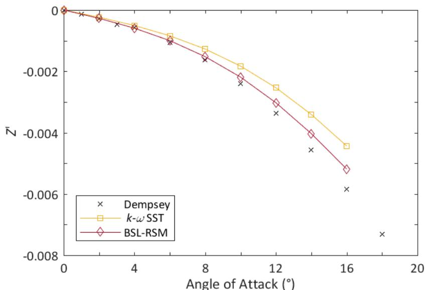
**Figure 6:** Variation of normal force with pitch angle for unappended Model 4621 hull.
