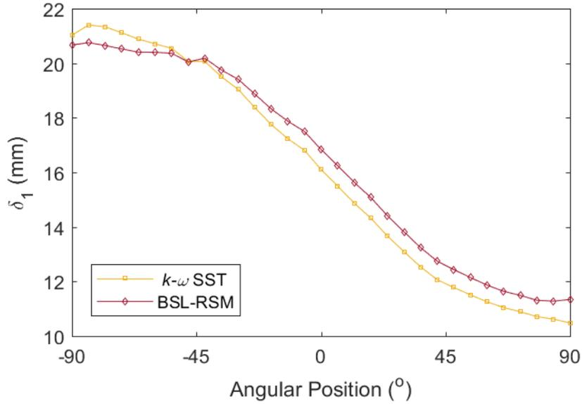
**Figure 9:** Azimuthal variation of the displacement thickness at  $x/L = -0.454$  of the unappended Model 4621 hull for  $k-\omega$  SST & BSL-RSM TCM.
