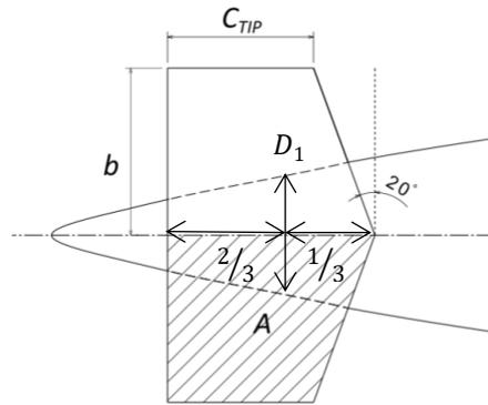
**Figure 2:** Plan view of Model 4621 afterbody showing a generic trapezoidal ACS with reference dimensions.
