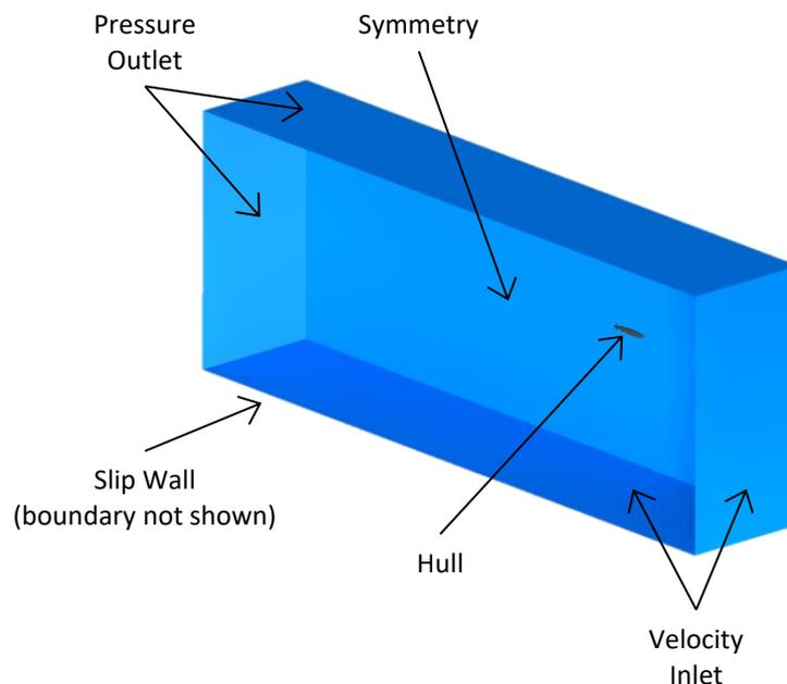
**Figure 3:** Fluid domain and boundary conditions
