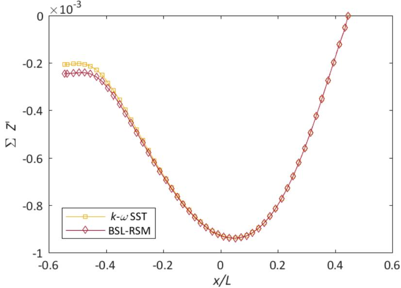
**Figure 8:** Cumulative summation (bow to stern) of the z-direction pressure force acting on the unappended Model 4621 hull.
