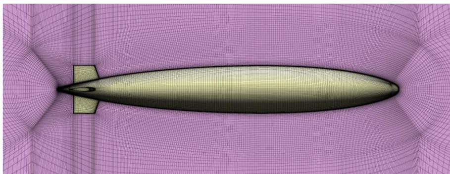
**Figure 4:** Surface mesh for the 11B appended Model 4621 hull and the symmetry plane mesh (every second gridline shown)
