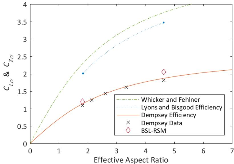
**Figure 10:**  $C_{Z,\alpha}$  for 3B & 11B appended Model 4621 hull.
