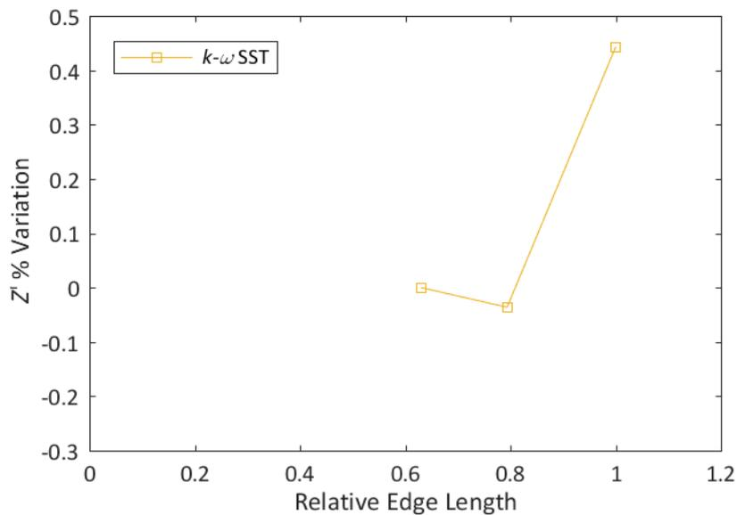
**Figure 5:** Percentage variation in normal force coefficient relative to finest grid
