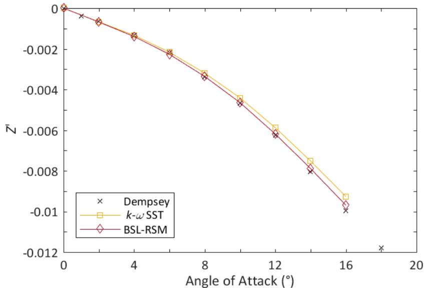
**Figure 7:** Variation of normal force with pitch angle for the 11B appended Model 4621 hull.
