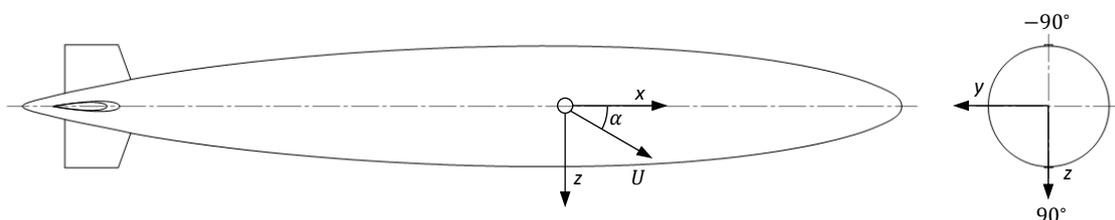
**Figure 1:** Appended Dempsey geometry and body fixed coordinate system with the origin at the centre of buoyancy.
